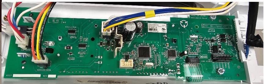
4. Locate the 4-pin coin connection AA4 or AA5. The coin drop harness for the main coin drop is the correct one to tap into.
